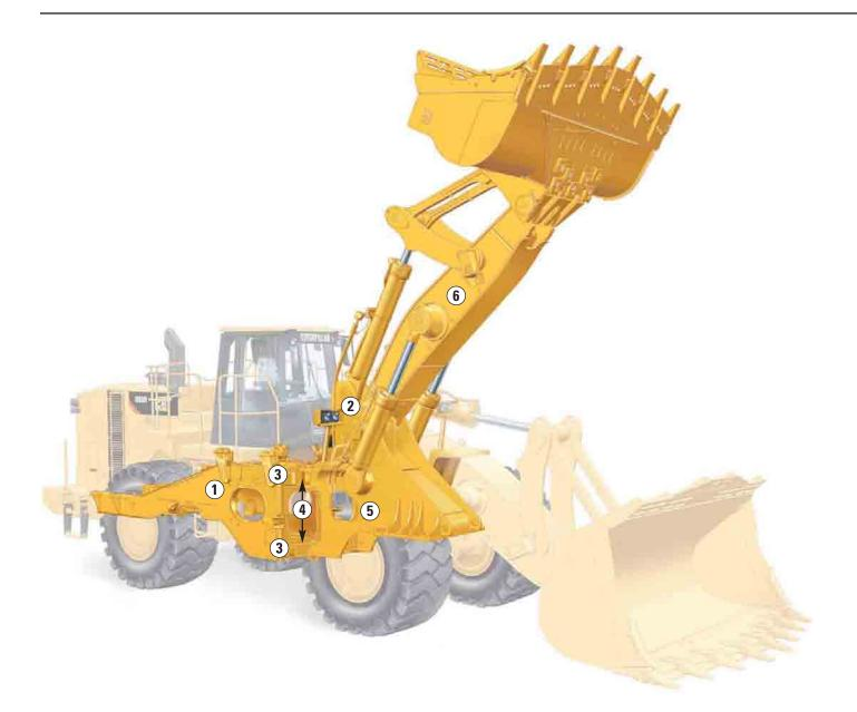
**Structures.** Combine the use of robotic welding and castings in critical high-stress areas. More than 90 percent of the 988H structure is robotically welded to provide highly consistent welds and increased strength. Castings are also used in several areas to increase strength by helping to spread the loads and reduce the number of parts.
