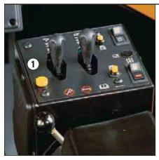
1 Electro-Hydraulic Control System. Increases hydraulic efficiency and enhances operator comfort through low-effort, fingertip controls. XT-3<sup>TM</sup> and XT-5<sup>TM</sup> hose along with reliable components reduce the risk of leaks and blown lines, helping protect the environment.
